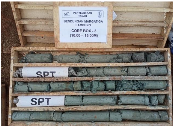
Figure 9 Core sample from boring activity at Margatiga Dam Project
