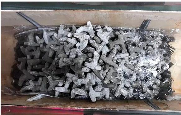
**Gambar 10** Uji Model Fisik *Breakwater* Dolos Skala 1:40
