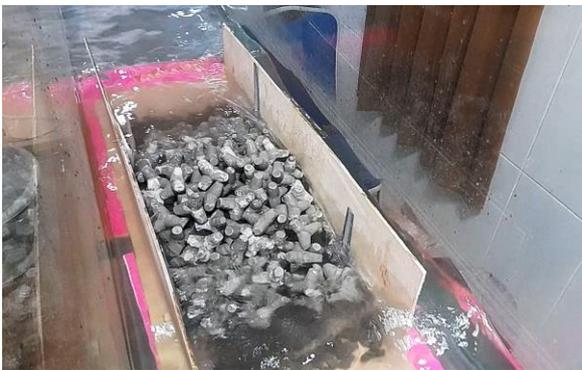
**Gambar 9** Uji Model Fisik *Breakwater* Tetrapod (Skala 1:40)
