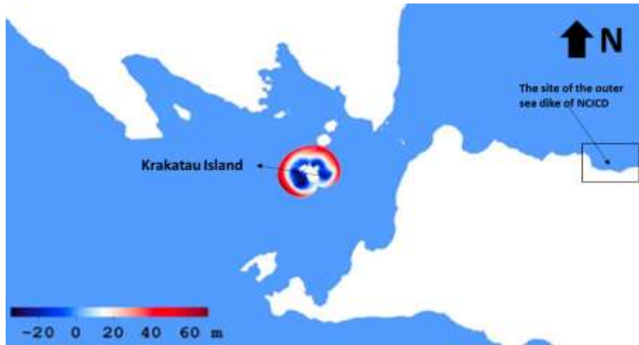
Figure 3 Increased water elevation induced by pyroclastic flow of Mount Krakatau: modified from Maeno and Imamura (2011)
