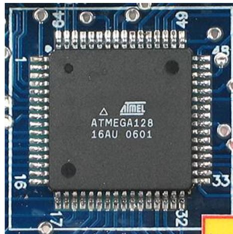
Gambar 7 Mikrokontroler ATMega128
